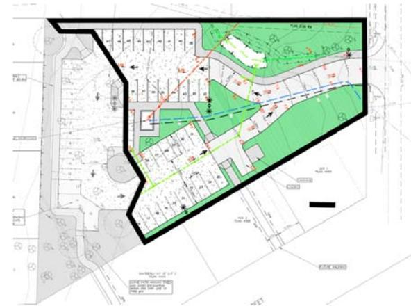
Phase 1 of the parking hub project provides 33 new parking spots in the downtown core. Construction will include drainage and storm pipe connections, relocating and servicing of the Tugwell Fields washroom, installation of electric vehicle charging stations, and access pathways. Phase 2 of the project will be considered in the future depending on demand.
